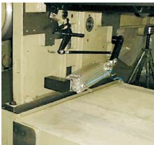
Verniciatrice Mailander: lama pneumatica Mailander coater: pneumatic scraper blade
