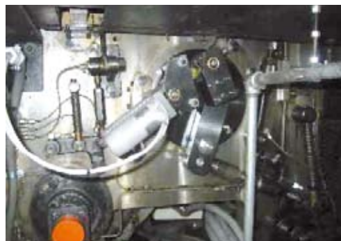
Crabtree Marquess: regolazione automatica pressioni Crabtree Marquess: automatic pressure setting
